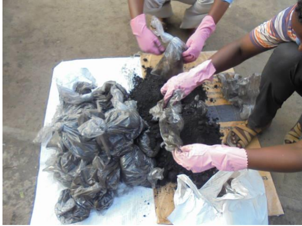
35. Once the vessel discharge was complete, all the samples per hold were combined to give a composite sample.
