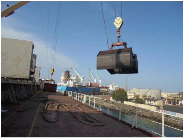
19. Empty crane grab after off-loading coal onto the quay.
