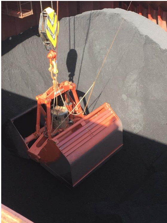
17. Crane grab collecting coal from hold 4.
