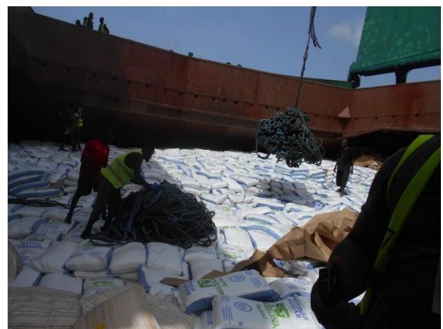
16. Slings lowered into hold.
