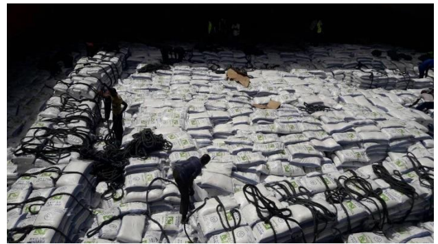
20. Slings prepared for discharge.
