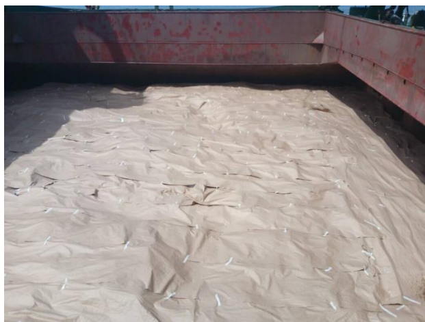
13. Cargo condition on arrival in Abidjan. Paper covering intact and no sign of water damage.
