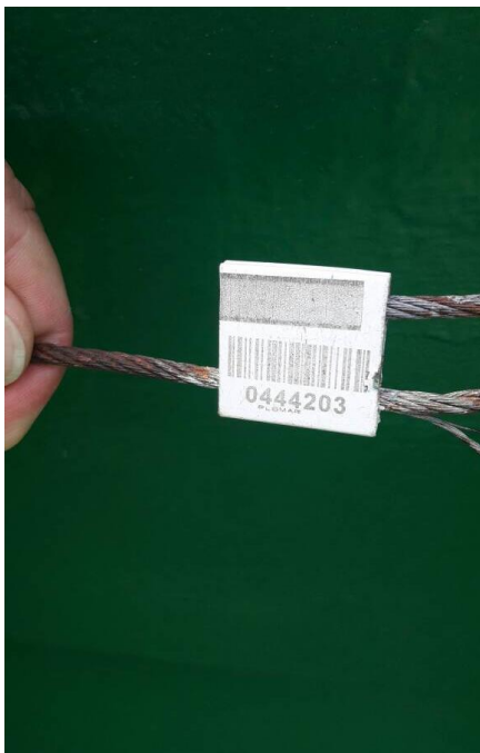
3. Hold 4 – Aft Access – Seal intact.
