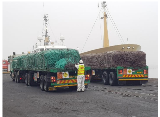
10. Loaded trucks covered with tarpaulin and secured with lashing prior to departure from the port.
