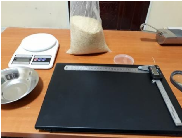
11. Tools used to analyse percentage broken of samples.
