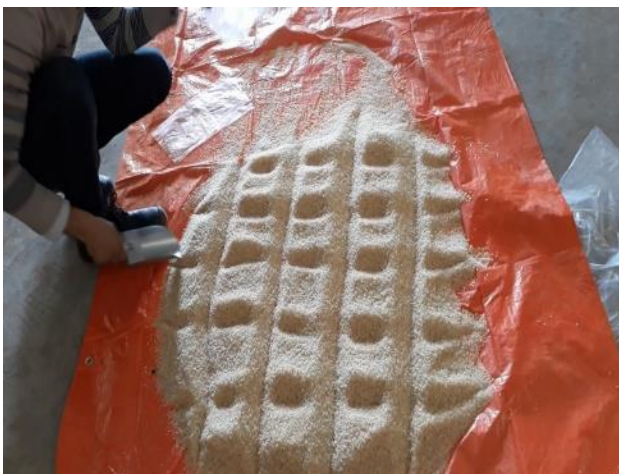
9. Mixing and dividing samples to get a representative sample.
