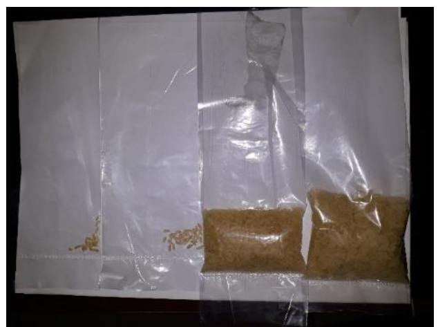
16. Sorting of damaged, red, yellow and broken kernels to be weighed.
