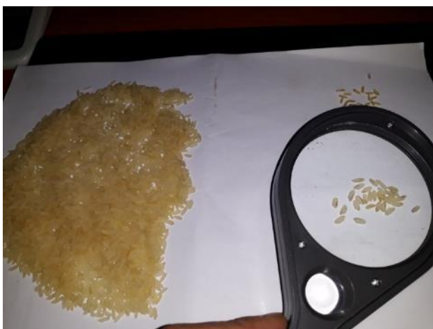
15. Visual inspection of the damaged, red, yellow and broken kernels.
