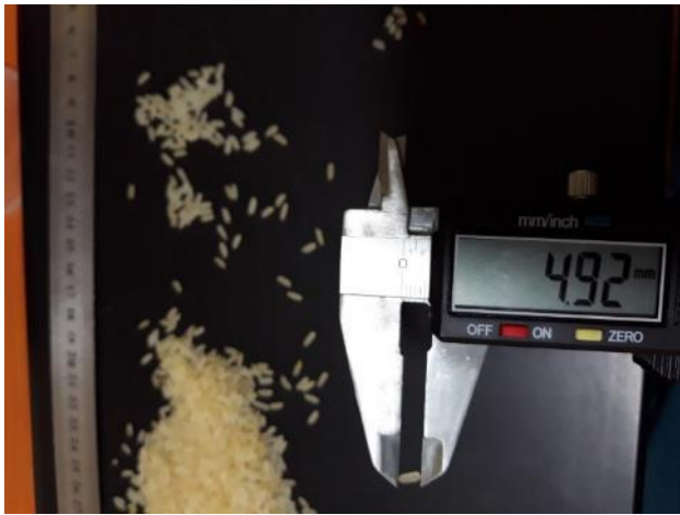
13. Checking average length of the grains.
