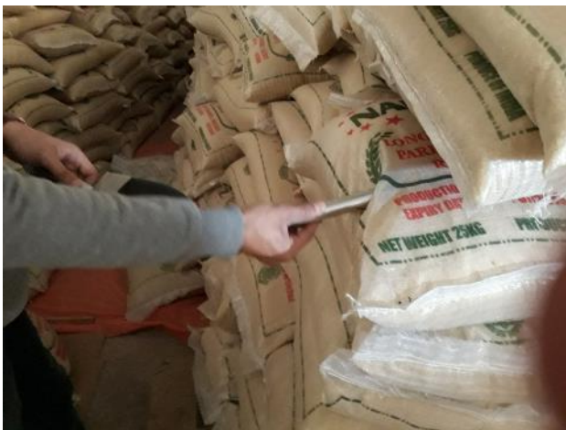
7. Sampling of goods using sample spear.
