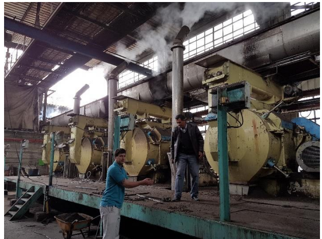
14. Vallis Egypt Country Manager, Jack Aylward and 4 Heat Compressors which turn the pulp into pellets.
