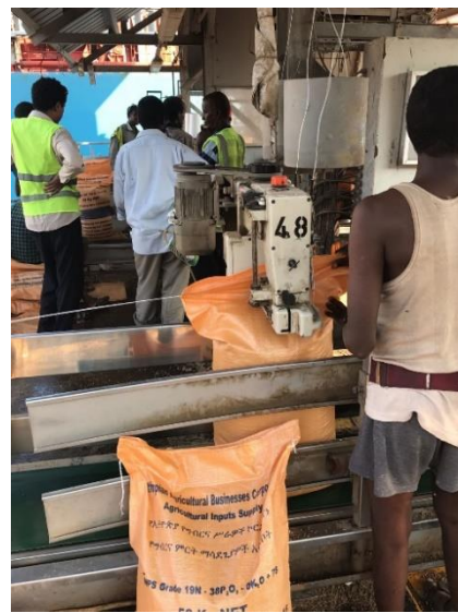
28. Bags being sewn shut on the bagging line.
