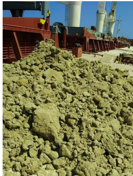
24. Caked cargo on deck to be removed by vessel.
