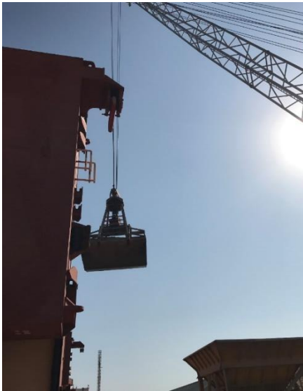
17. Cargo discharged from the vessel using grabs attached to the ship's crane.
