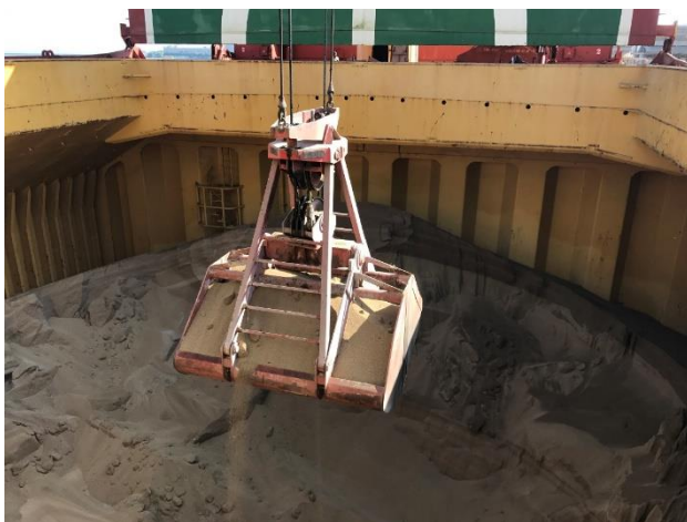
13. Cargo being lifted using grabs.
