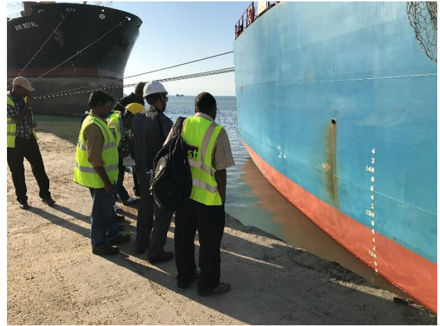
4. Draft survey underway.
