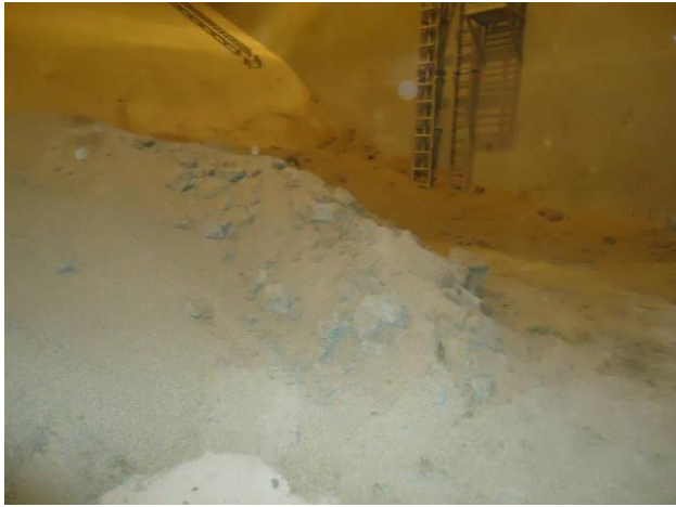
21. Water ingress discovered in the hold.
