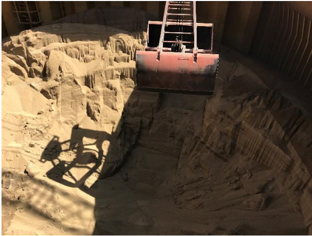
15. Additional view of grabs being used to discharge cargo.
