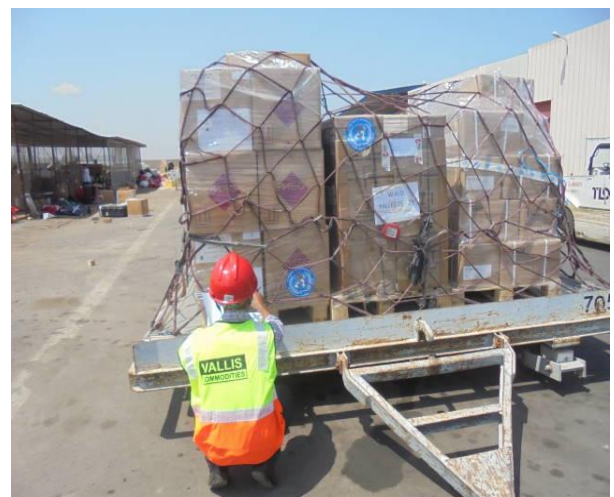
4. Pallets placed on cargo trolley and wrapped in netting to be loaded onto aircraft.
