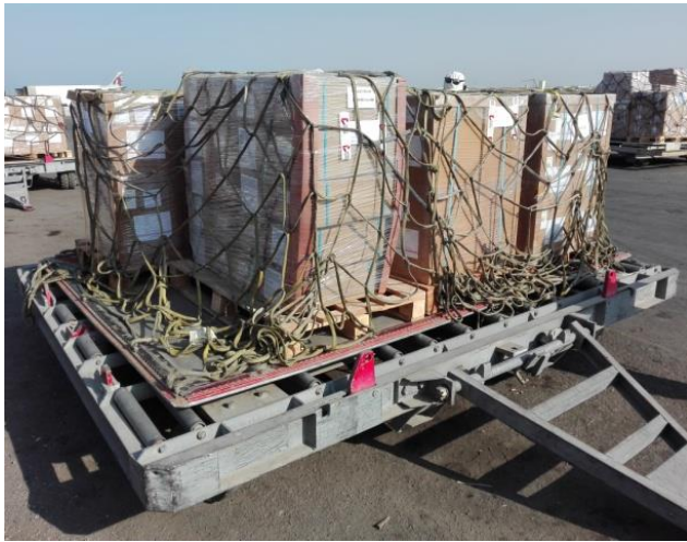
5. Pallets placed on cargo trolley and wrapped in netting to be loaded onto aircraft.
